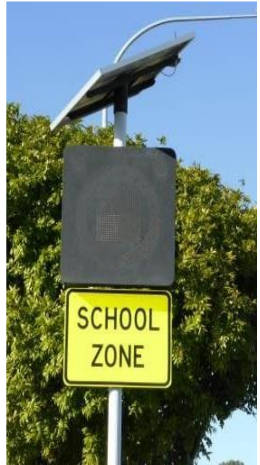
When the zone is not activated, the electronic sign looks black so as not to confuse motorists.
